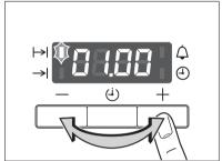
After approx. 5 seconds the display returns to showing the current time. The function indicator Cook time  $\bowtie$  lights up.
